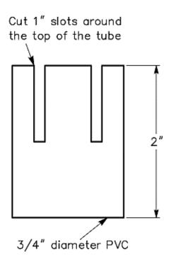
Figure 3—Make two clamps by cutting 1-inch slots into two 2-inch long, <sup>3</sup>/4-inch diameter PVC tubes. When you tighten the steel hose clamps around these slots, they'll apply firm pressure to the PL-259 connectors, holding the ground planes in place.
