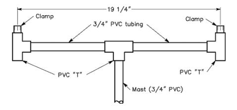
Figure 2—Assemble the boom using <sup>3</sup>/<sub>4</sub>-inch diameter PVC tubing and Ts. Note that the distance is 19<sup>1</sup>/<sub>4</sub> inches between the center of one PVC "end T" and the other.
